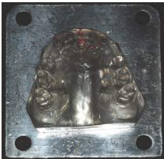
Figure 1 The master model screwed onto the impression carrier of the testing device.
