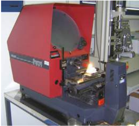
Figure 7 The profile projector used for the measurements.
